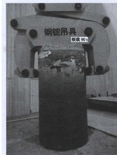
图 3 60 t X2CrNiMo18-12 奥氏体不锈钢电渣锭形貌 Fig. 3 Morphology of 60 t ESR ingot of austenite stainless steel X2CrNiMo18-12
